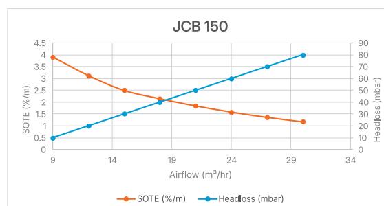
Standard Oxygen Transfer Efficiency (SOTE) and Headloss for JCB 150 Performance
