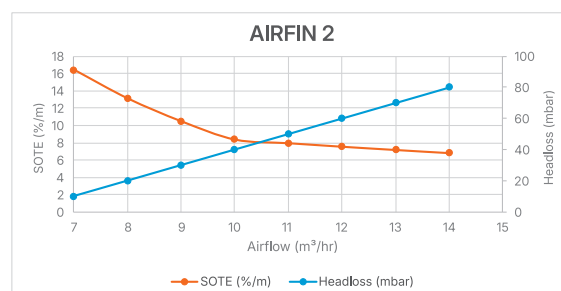
Standard Oxygen Transfer Efficiency (SOTE) and Headloss for AIRFIN 2 Performance
